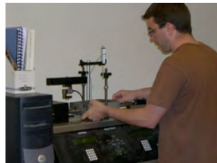
(b) student performing a direct shear test
