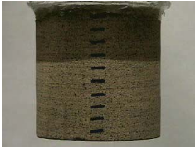
Figure 3: Ohio sandstone during wicking test series II
