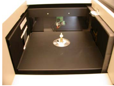
(b) photograph of the inside of the scanner with specimen mounted in the center
