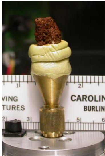
Figure 17: Concrete specimen imbibed with 21 drops of iodine solution
